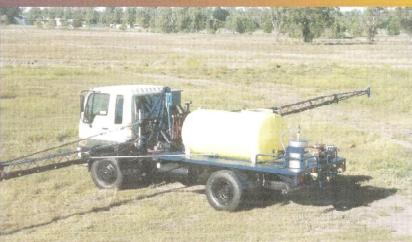
The trucks are fitted with Davey twin impellor firefighter pumps, plumbed for loading and spraying. The rear step gives access to the large tray, with enough room to mix and store chemicals, and accessories.
