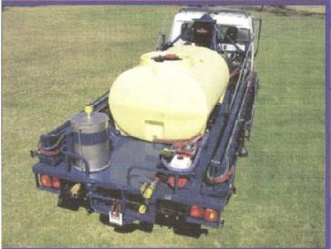
Plumbing is simple to reduce the risk of chemical contamination, using high quality, chemical resistant hose and standard sized fittings.
