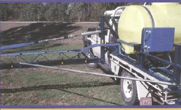
A wide fold down rear step, with handrail, gives safe access to the rear work area. A sensible layout of camlock fill points, filters and taps allow the operator to fill quickly and efficiently.
