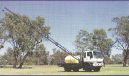
Monitors are factory fitted to be close at hand, so all functions are easily reached. Sprayers are fitted with an engine stop in the cab.
