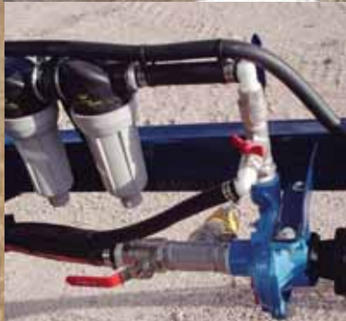
Pressure Filters are rated at 200psi
